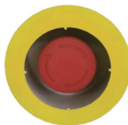
Figure 5.7 After Crushing of Emergency Stop Button
